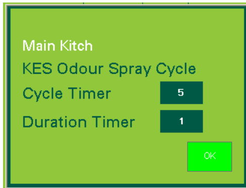
Enviro odor spray cycle and duration timers. Figure 26
