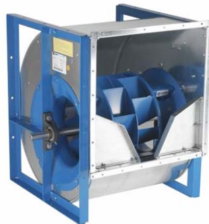
A KESF DWDI fan. Correct rotation for this fan arrangement looking into the end shown above is clockwise Figure 25
