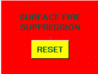
Typical fault displayed on Dashboard screen after surface fire suppression activates.
