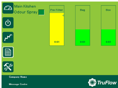
Enviro filter status screen shown on kitchen mounted Truflow panel Figure 10
